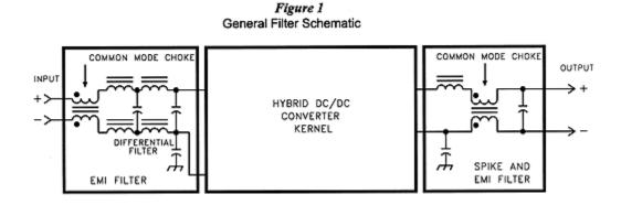
Within the DC-DC Converter, conducted emissions can be differential mode or common mode. Differential mode emissions appear primarily on one input power lead, whereas common mode emissions appear on both because of the nature of the sources that generate the emissions, differential noise is more common below 1-2 MHz, where common mode noise is more prevalent at higher frequencies.
